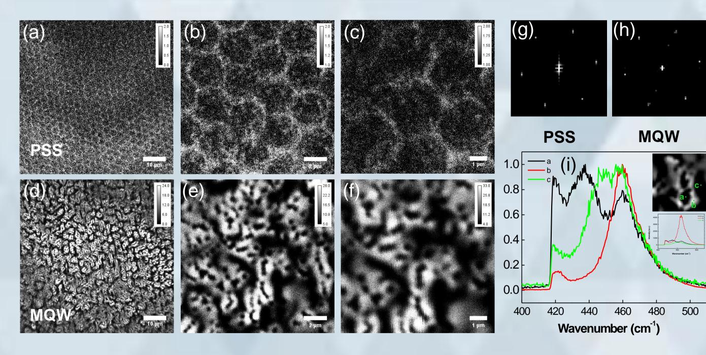
(a)-(c): Reflectivity mapping of PSS, and (d)-(f): PL mapping of MQW in different scales. (g),(h): Fast Fourier transform (FFT) of images (a) and (d) reveal that PL patterns in MQW is directly correlated with the structural pattern in PSS. The PL mapping of MQW layer can be divided into three areas: v-pit, bright area, and dark area. Normalized spectra correspond to these three areas as shown in (i).
