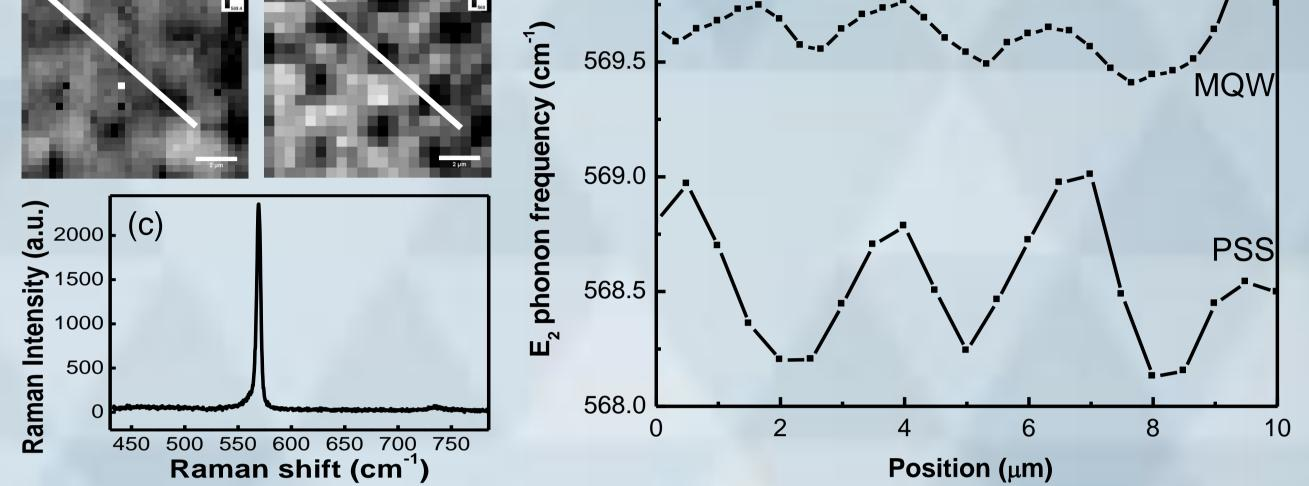
(a), (b): The mapping of  $E_2$ (high) phonon peak position of MQW and PSS, where the peak position is determined by Gaussian peak fitting. (c) shows a representative Raman spectrum inside the sample. (d) Plot of peak position variation along the green lines shown in (a) and (b).
