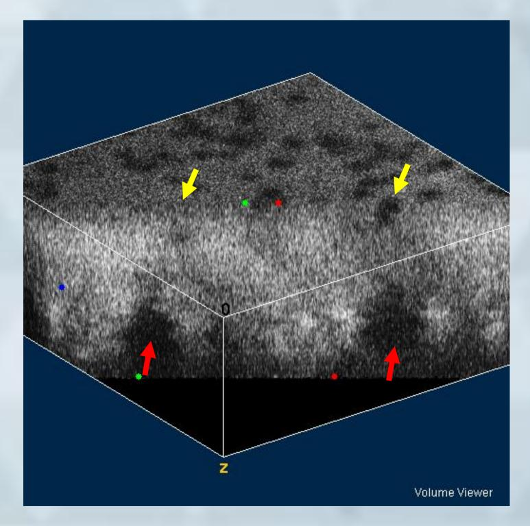
The 3D reconstruction of axial  $E_2(high)$  Raman mapping. The two lower dark areas (red arrows) correspond to the tip of two protruded patterns in PSS. From this threedimensional image plot, the origin of the two vpits (yellow arrows) in MQW can be traced to the two tips in PSS.
