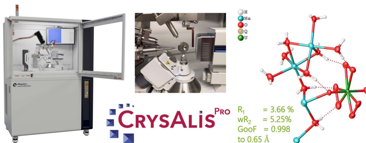
Figure 1. Na 4 O 17 U under high pressure: Hardware and software in Synergy.
