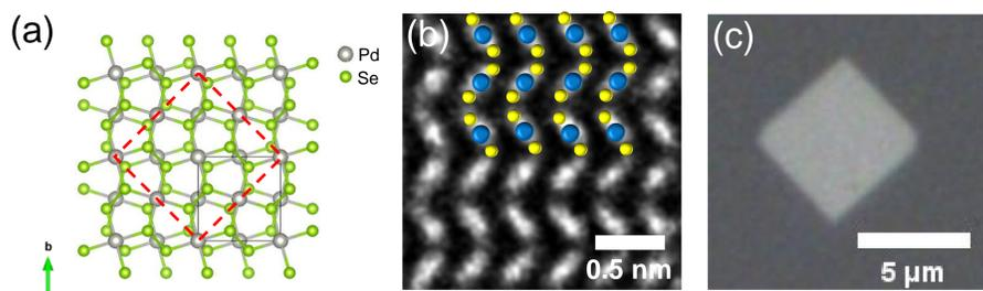
**Figure 1.** (a) Top view of the crystal structure of 2-layer (2L) PdSe<sub>2</sub> showing a puckered pentagonal configuration. (b) Atomic resolution structure of 2L PdSe<sub>2</sub> crystal revealed by TEM image. Inset showed atomic model of the corresponding TEM image. (c) Optical image (OM) of CVD grown PdSe<sub>2</sub> flake on sapphire substrate.
