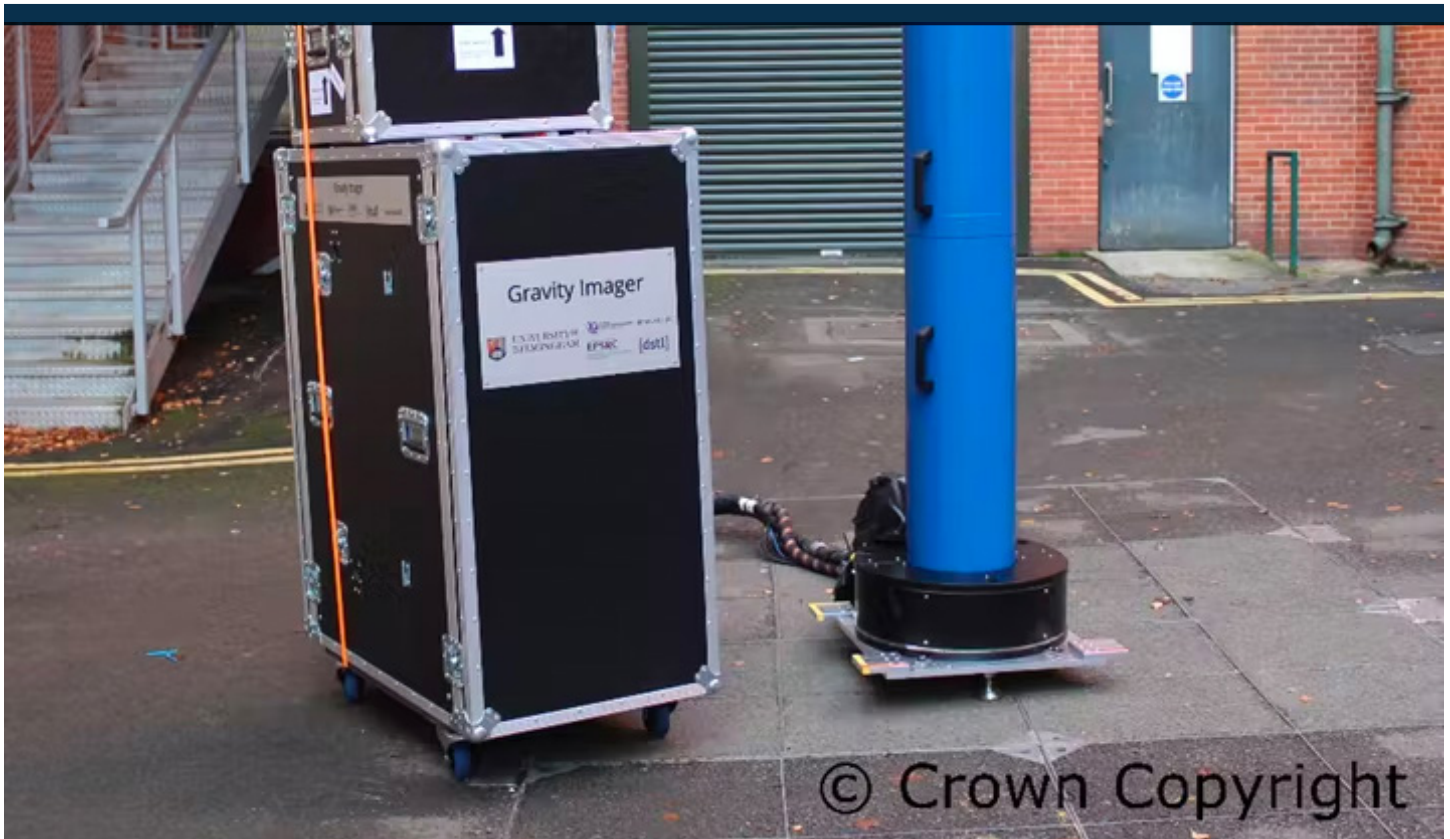
FIGURE 1. The quantum technology-based gravity gradient sensor.
