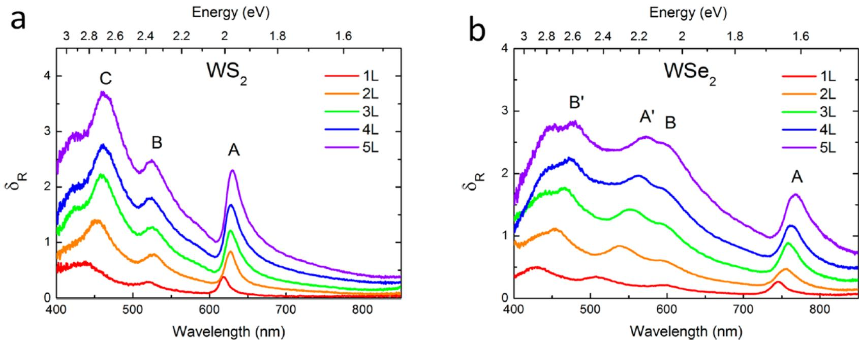
Figure 1. Differential reflectance spectra of mechanically exfoliated (a) 2H-WSe<sub>2</sub> and (b) 2H-WSe<sub>2</sub> flakes consisting of 1–5 layers. The peaks are labeled according to the convention proposed by Wilson and Yoffe.<sup>22</sup>
